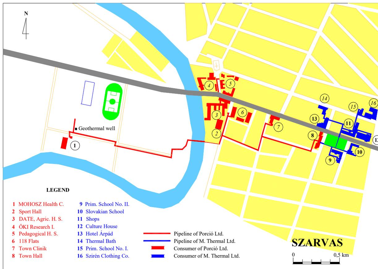
Figure 3. Site plan of the Szarvas geothermal utility
