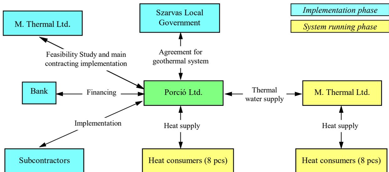
Figure 2. Construction of agreements for the Szarvas geothermal utility
