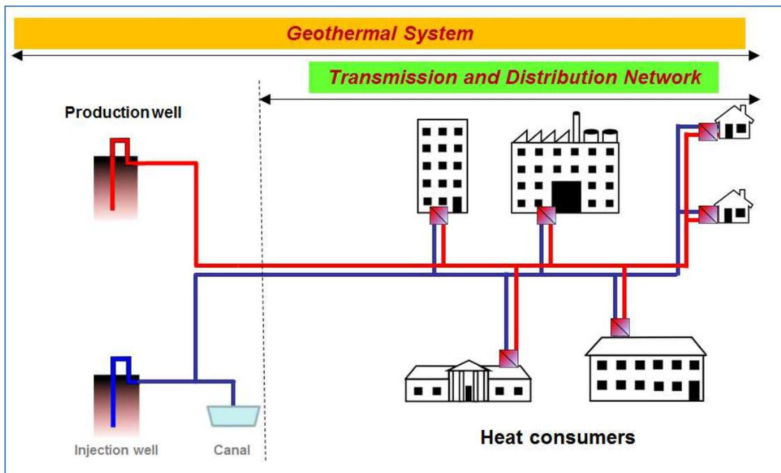
Figure 3 Scheme of geothermal public utilities
