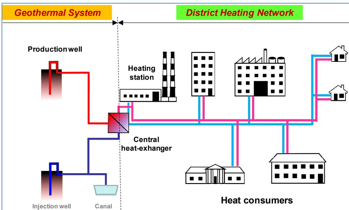
**Figure 2 Scheme of geothermal based district heating**
